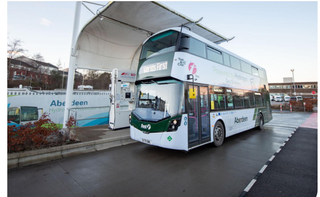
Figure 13: 350 bar hydrogen nozzle connected to vehicle during refuelling. During this process, the bus is earthed by an earthing cable to reduce static electricity.
