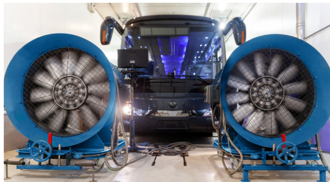
Figure 3: A Yutong TCe12 electric coach being tested over the UK Bus Cycle on a rolling road (chassis dynamometer) under controlled lab conditions to qualify for capital grant funding under Transport Scotland’s Scottish ULEB Scheme (Credit Yutong).
