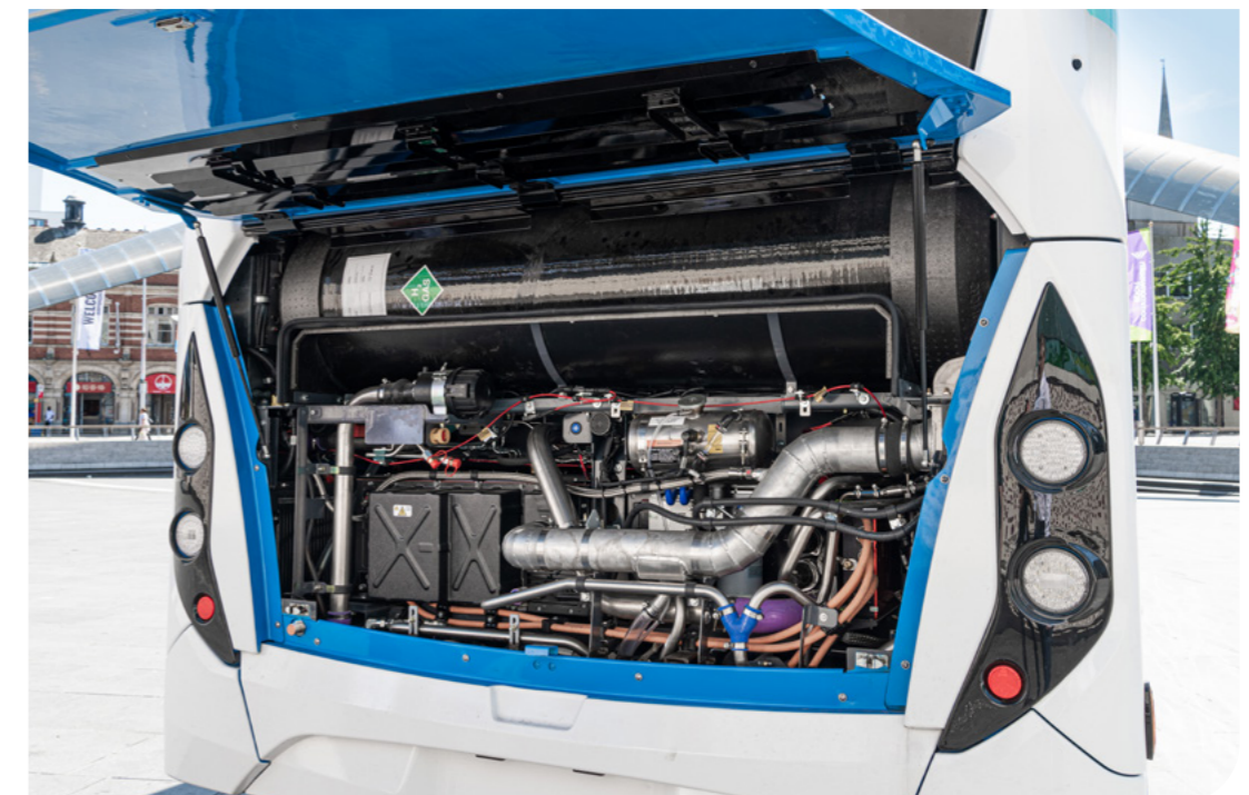
Figure 11: Engine bay of Alexander Dennis Enviro400FCEV highlighting packaging layout of fuel cell and hydrogen tanks
