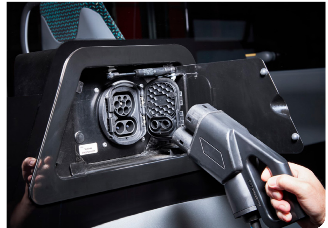
Figure 7: Combined Charging System 2 (CCS2) plug and vehicle interface.
