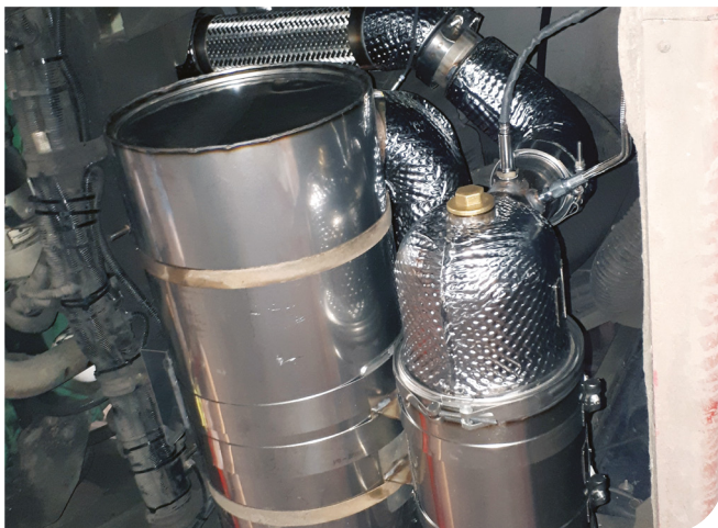
Figure 6: Proventia/Excalibre Technologies NOxBUSTER™ SCR System fitted to ADL E200 Euro V Bus
