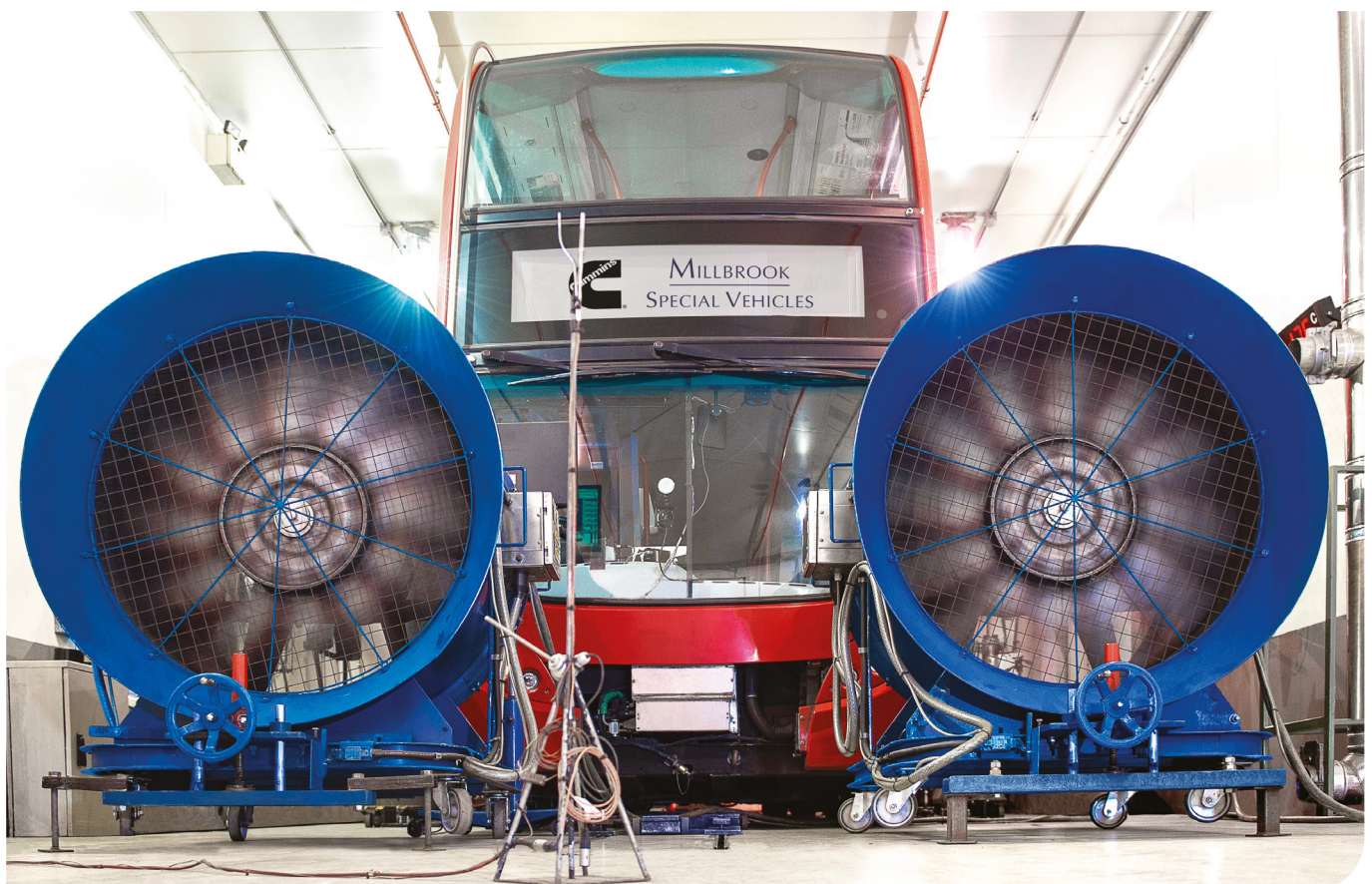
Figure 12: An ADL E400 undergoing testing following Repower with a Cummins Euro VI Phase C 6.7 litre engine by Millbrook Special Vehicles
