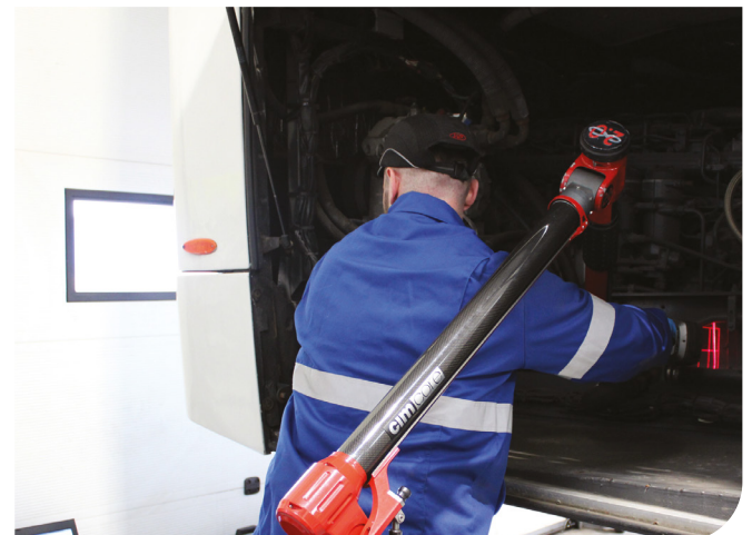
Figure 7: Technician creating 3D digital image of internal body of a coach using a laser system to identify available space for SCR system (courtesy of Eminox)
